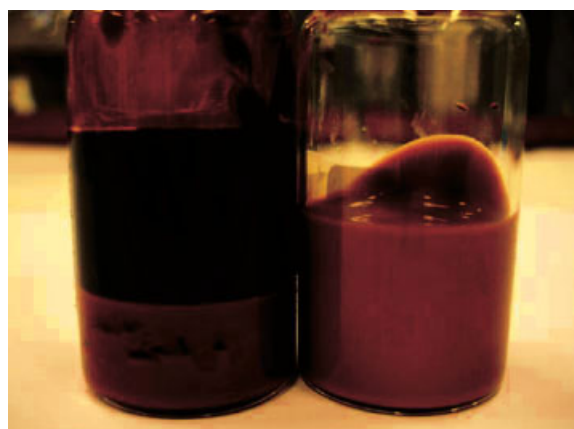
Figure 8 Pictures of the emulsions: left sample at 80% protonation after 2 month storage; right sample at 50% protonation after 1-year storage. (PK30/mPK30 = 2,500 rpm, 50°C, 1 h). [Color figure can be viewed in the online issue, which is available at www.interscience.wiley.com .]
